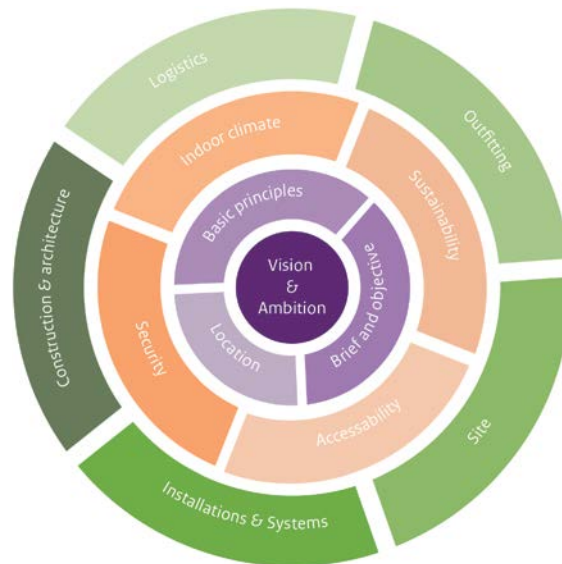
Figure 4 Diagram depicting the different layers contained in an SoR. Image: Bart Ankersmit
